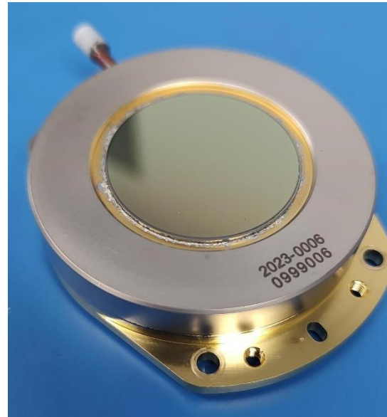
Fig. 10. Photograph of a complete package. Cover diameter is 56.8 mm.
