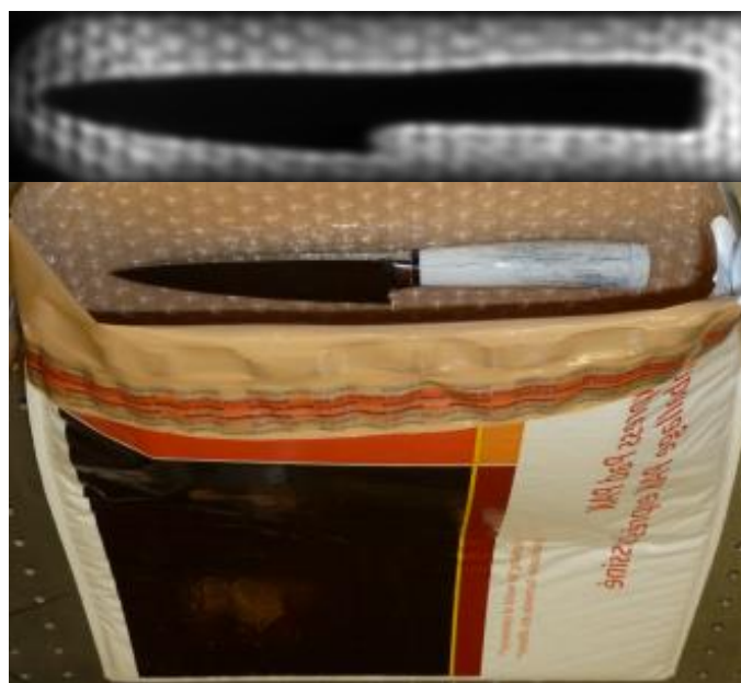
Fig. 5. THz mosaiced image taken at 432 \mu\text{m} of a knife seen through a padded (with bubble wrap) mailing envelope (top) visible image showing the knife hidden inside the padded envelope (bottom).
