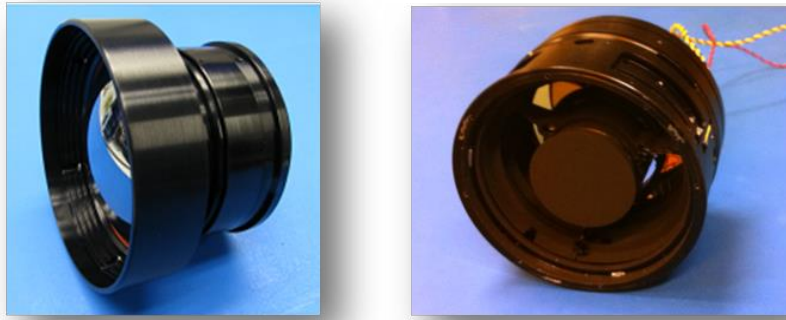
Fig. 2. Refractive (left) and catadioptric (right) THz objectives
