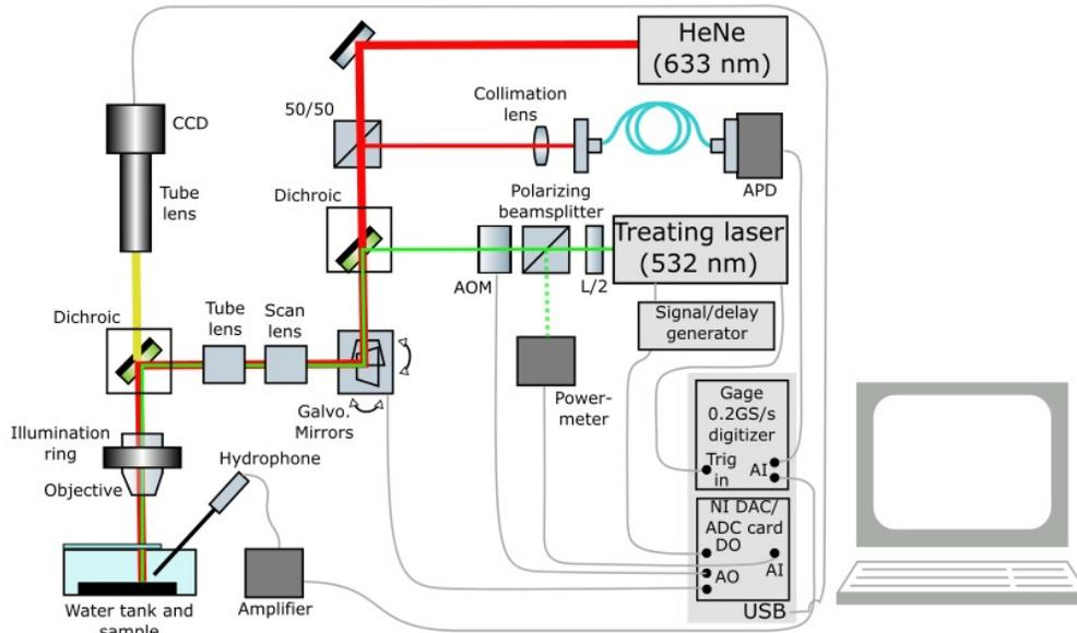
Figure 1. Laser therapy with photoacoustic dosimetry experimental setup. AOM: Acousto-optic Modulator and APD: Avalanche Photodiode.
