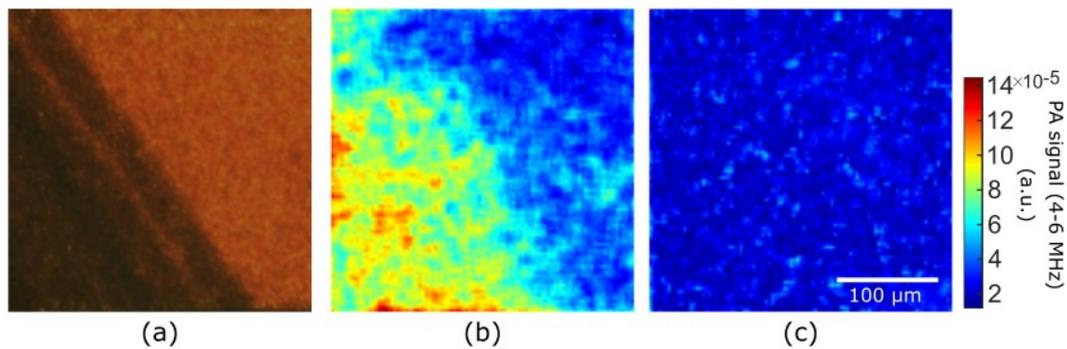
Figure 3. a) CCD microscopic image of a non-uniform sample (black ink was applied in the lower left corner and red ink was applied in the upper right corner). Corresponding PA image of the sample imaged on the left (b) and PA feedback image obtained with treatment titration (c). Note that treatment effect is uniform over the sample despite spatial absorption variations. Scale bar applies to (a), (b) and (c). PA signal scale applies to (b) and (c).
