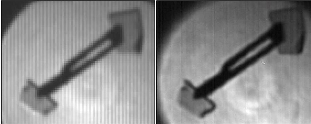
Figure 5: Terahertz images of the same scene captured with a 160x120 pixel imager with 52  $\mu\text{m}$  pixel pitch pixel.
