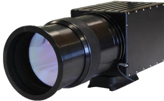
Figure 1: HRXCAM-16K an infrared camera with a catadioptric optics that can oversample the images with a microscan of 16 x 16 pixels yielding images of 16348 x 12288
