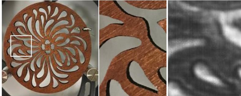
Figure 6: Terahertz image in transmission of a wooden object captured at a wavelength 580  $\mu\text{m}$ .
