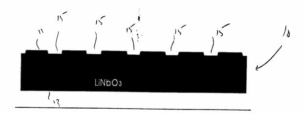
FIG. 1 Periodically-etched (diced, polished) LiNbO3 crystal.
