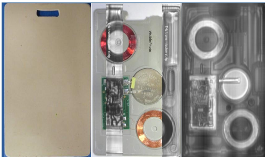
Visible image of opened card with THz transmission strips
