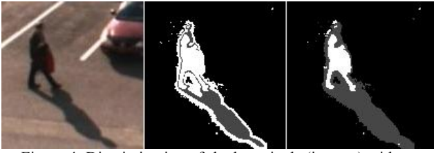
Figure 4: Discrimination of shadow pixels (in gray) with an association volume symmetrically centered on a distribution (center) and with the proposed volume ( \tau_{Y,up}=1 )(right).
