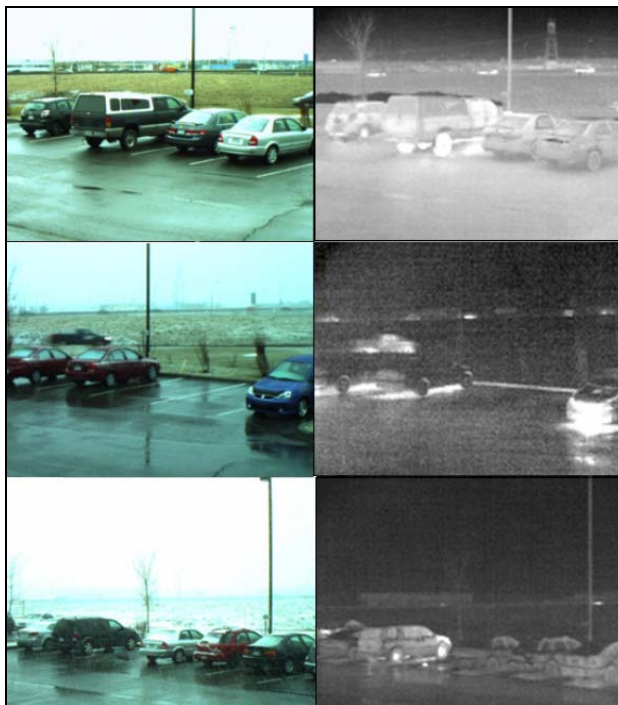
Fig. 1: Visible and LWIR images during slight overcast (top), strong wind and rain (middle) and snow (bottom).
