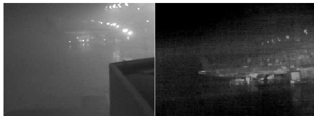
Fig. 2: Visible (left) and LWIR (right) images in thick fog (courtesy of Ottawa airport and Searidge Technologies, Ottawa, Canada).
